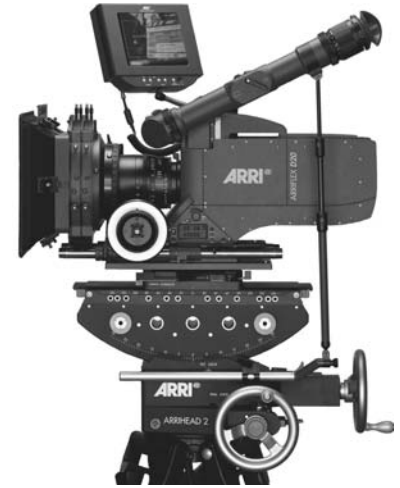
An Arriflex D-20 digital video camera. The camera features a Super 35-sized CMOS imaging grid, allowing it to use all the same PL-mount lenses and accessories as an Arri film camera. It also provides a traditional optical viewfinder and a color video monitor (courtesy ARRI Group, www.arri.com ).
